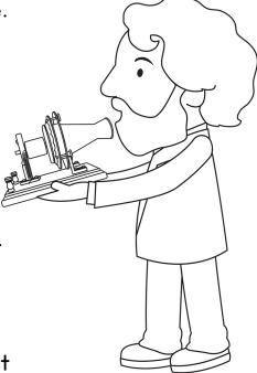
Bell's first telephone was very simple. It had a transmitter and a receiver. The transmitter turned the sound of your voice into electric signals. These signals traveled through a wire to the receiver. The receiver turned the signals back into sound so the other person could hear your voice. It was a very clever invention!
